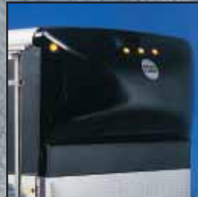
Aerodynamic Nose Cone®
